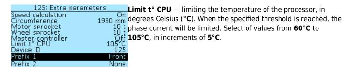
**Device ID** — setting the Controller number in the CAN network. This number is displayed in the menu section **Settings** > **Devices** in front of each device that is connected to the network using the **LEVCAN** protocol. If, by default, your device number is **0**, we recommend changing it to another number for the correct firmware update.
