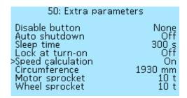
**Speed calculation** — enabling speed calculation in the Controller. Useful for multi-motor configurations, you can turn off the speed calculation on some motors. Select of values **On** and **Off**. **Circumference** — wheel circumference, in millimeters (mm). Select of values from **Omm** to **3000mm**, in increments of **5mm**. To calculate the circumference, you can use online calculator.
