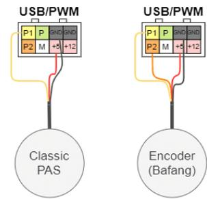
Controller 6F v1.0 pinout
