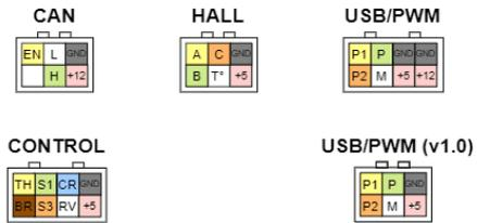
Controller 6F v1.6 pinout
