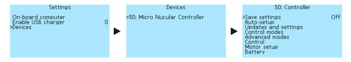
After configuring the battery, you need to run Auto-setup in the **Controller > Auto-setup** menu section. Ensure that the phase and battery wires are well contacted and insulated before running
