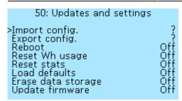
**Import config.** — loads the settings from the file **NCconf.cfg** - **NCconf9.cfg** up to a maximum of 9 different configurations, choosing a file number from 1 to 9. After a successful import, error messages may appear in the message, this means that not all the settings have been imported. In this case, it is advisable to check the downloaded settings with the original file by opening it in Notepad.
