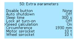
**Speed calculation** — enabling speed calculation in the Controller. Useful for multi-motor configurations, you can turn off the speed calculation on some motors. Select of values **On** and **Off**.
