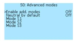
To activate the control modes, select **Controller > Advanced modes > Enable add. modes** and to set **On**.
