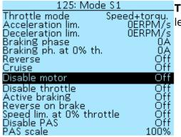
Throttle mode — selection of the operating mode of the throttle operating mode of the throttle lever, read more in the section Throttle control mode setup.
