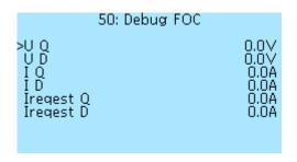
**U Q** — Q-axis voltage, in volts (**V**).
