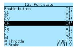
In the section **Controller** > **I/O configuration** > **Port state**, you can check input activation when contact shorted to GND. When a signal is applied, the value will change from **Off** to **On**. Below in the
