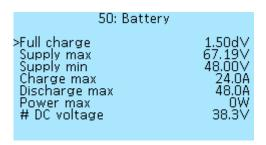
**Full charge** — delta voltage relative to the maximum, at which when the controller is turned on, will reset the watt-hour consumption, in volts (**dV**). This setting resets the **From charge statistics** when the Controller is turned on. Select values from **0.00 dV** to **10.00 dV**, in increments of **0.3 dV**.
