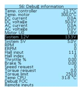
**Temp. controller** — temperature of the Controller, in degrees Celsius (°C).
