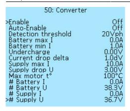
**Enable** — turn on the converter mode and start charging. Select of values **On** and **Off**.
