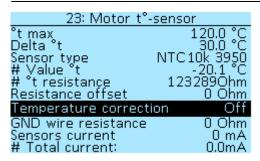
**°t max** — maximum electric motor temperature, in degrees Celsius (°C). Select of values from **50°C** to **200°C**, in increments of **1°C**.
