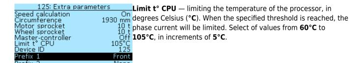
**Device ID** — setting the Controller number in the CAN network. This number is displayed in the menu section **Settings** > **Devices** in front of each device that is connected to the network using the **LEVCAN** protocol. If, by default, your device number is **0**, we recommend changing it to another number for the correct firmware update.
