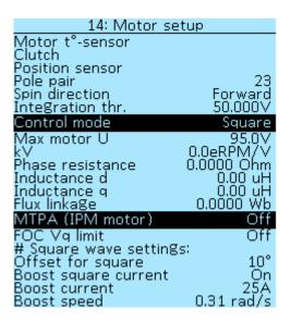
**Pole pair** — the number of magnetic pole pairs of the rotor of the electric motor determines the speed at which the motor shaft will rotate. This parameter is used to calculate RPM and speed. For a
