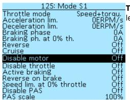
Throttle mode — selection of the operating mode of the throttle Speed+torqu. lever, read more in the section Throttle control mode setup.
