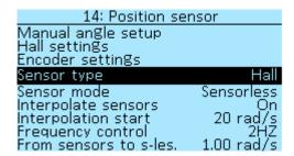
**Sensor type** — Parameter needs reboot if manually changed. There are currently two types of sensors available:
