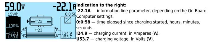
**The indication in the middle** is the temperature of the motor and the controller, respectively, in degrees Celsius (°C).
