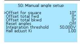
**Offset for square** — additional shift for square wave mode, in degrees (°). Select of values from -30° to 30°, in increments of 1°.
