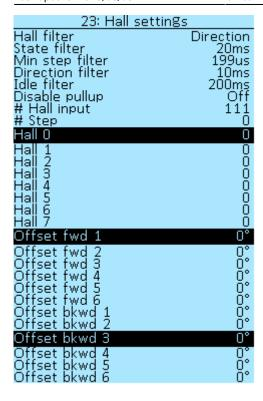
**Hall filter** — enable or disable the filter in the direction of rotation, select the **Direction** and **OFF** values.
