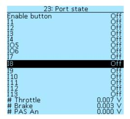
In the section **Controller** > **I/O configuration** > **Port state**, you can check input activation when contact shorted to GND. When a signal is applied, the value will change from **Off** to **On**. Below in the menu items **# Throttle** and **# Brake** you can see the voltage on the throttle and brake levers, respectively.
