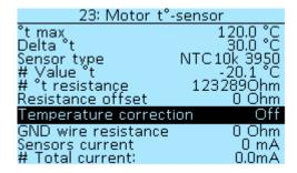
**°t max** — maximum electric motor temperature, in degrees Celsius (°C). Select of values from **50°C** to **200°C**, in increments of **1°C**.
