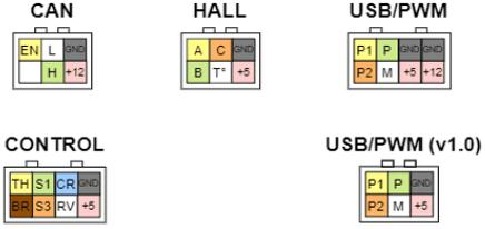
Controller 6F v1.6 pinout
