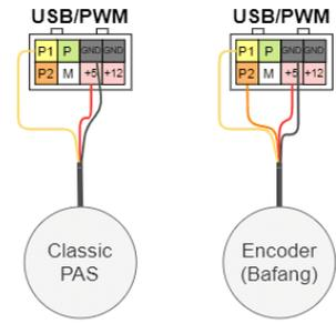
Controller 6F v1.0 pinout
