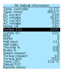
**Temp. controller** — temperature of the Controller, in degrees Celsius (°C).
