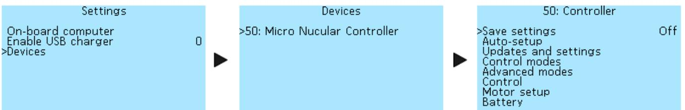
After configuring the battery, you need to run Auto-setup in the **Controller > Auto-setup** menu section. Ensure that the phase and battery wires are well contacted and insulated before running
