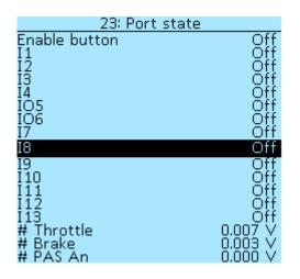
In the section **Controller** > **I/O configuration** > **Port state**, you can check input activation when contact shorted to GND. When a signal is applied, the value will change from **Off** to **On**. Below in the menu items **# Throttle** and **# Brake** you can see the voltage on the throttle and brake levers, respectively.
