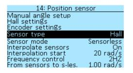
**Sensor type** — Parameter needs reboot if manually changed. There are currently two types of sensors available:
