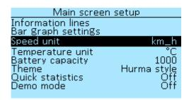
**Speed unit** — in kilometers per hour (**km\_h**) or in miles per hour (**mph**). **Temperature unit** — in degrees Celsius (°**C**) or degrees Fahrenheit (°**F**).
