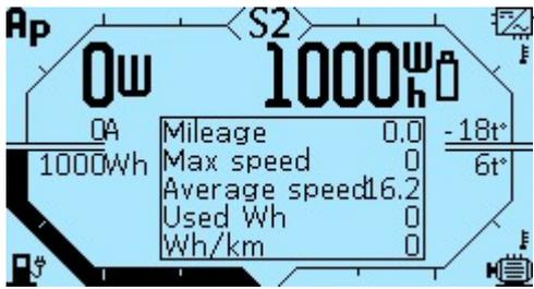
You can choose to display several types of statistics: **General, User, Trip, From charge**. For a detailed description, see the **Statistics** section. The main screen displays five parameters:
