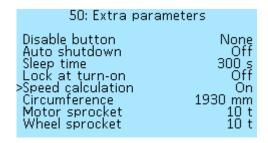
If selecting a value **Display** the speed will be determined from an external sensor, which is used, for example, in a bicycle computer. The speed sensor must be connected according to the diagram to the **SPEED** connector on the rear panel of the On-board computer. After setting the Display value and connecting the speed sensor, you must specify the wheel circumference in millimeters in the **On-board computer > Data source menu**.
