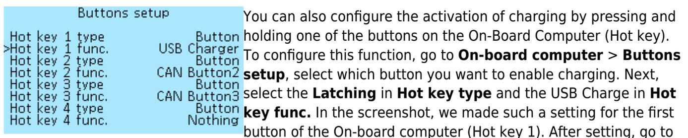
the **On-board computer** > **Save** and save. Done. USB charging can now be turned on/off by pressing and holding the first button of the On-Board Computer when the main screen is displayed.
