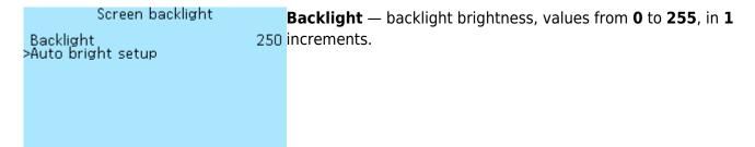
If desired, you can enable automatic screen brightness adjustment using the light sensor in the menu **On-board computer** > **Screen backlight** > **Auto bright setup**.
