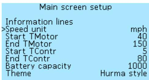
**Start TMotor** — minimum displayed motor temperature in degrees Celsius (°C), values from **5°C** to **250°C**, in **5°C** increments.
