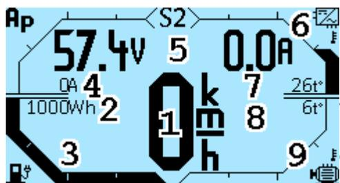
1. Speedometer or fast statistics, when the speed is zero.
