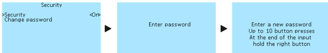
**Security** — enabling the password request function when starting the controller. Select **Off** and **On**. **Change password** — changing the default password.
