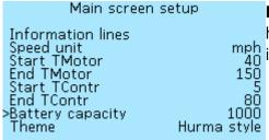
**Battery capacity** — the energy stored by the battery, in Watthours (W\*h), the values from **5** W\*h to **10000** W\*h, with increments of **5** W\*h.
