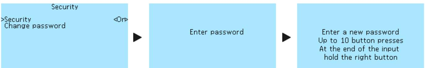
**Security** — enabling the password request function when starting the controller. Select **Off** and **On**.
