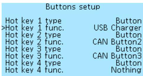
You can also configure the activation of charging by pressing and holding one of the buttons on the On-Board Computer (Hot key). To configure this function, go to **On-board computer > Buttons setup**, select which button you want to enable charging. Next, select the **Button** in **Hot key type** and the USB Charge in **Hot key func.** In the screenshot, we made such a setting for the first button of the On-board computer (Hot key 1). After setting, go to
