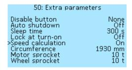
If selecting a value **Display** the speed will be determined from an external sensor, which is used, for example, in a bicycle computer. The speed sensor must be connected according to the diagram to the **SPEED** connector on the rear panel of the On-board computer. After setting the Display value and connecting the speed sensor, you must specify the wheel circumference in millimeters in the **On-board computer > Data source menu**.
