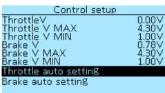
ThrottleV — current voltage of the throttle grip connected to the On-board computer, in volts ( $\mathbf{V}$ ).
