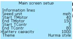
**Battery capacity** — the energy stored by the battery, in Watthours (W\*h), the values from **5** W\*h to **10000** W\*h, with increments of **5** W\*h.
