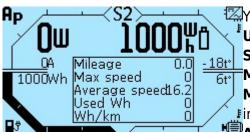
You can choose to display several types of statistics: **General**, User, Trip, From charge. For a detailed description, see the Statistics section. The main screen displays five parameters: Mileage — mileage in kilometers (km) or in miles (mi). Max speed — maximum speed, in kilometers per hour (km/h) or in miles per hour (mph).
