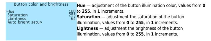
Also in this menu, you can enable automatic adjustment of the brightness of the buttons using the light sensor located on the front panel of the On-board computer. Menu **On-board computer > On-board computer settings > Button color and brightness > Auto bright setup**.
