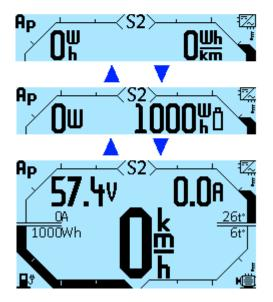
List of parameters available for display: **Nothing** — parameter is not displayed. **Voltage** — battery voltage, Volts (**V**). **Current** — battery current, Amperes (**A**). **Phase current** — phase current, Amperes (**A**). **Watts** — electric motor power, Watts (**W**). **Unused Wh** — remaining battery capacity, Watt-hours (**Wh**). **Used Wh trip** — energy consumption per trip, Watt-hours (**Wh**).
