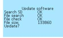
To update, download the firmware file to the root directory of the microSD card with Fat/Fat32 file system. Insert the card, with the contacts on top, into the connector on the On-board Computer. This can be done without turning off the On-board computer, but in this case, you must exit the **Update software** menu and reenter. After that, the On-board computer will detect the microSD card, display the **File size** in bytes and the menu item **Update**?
