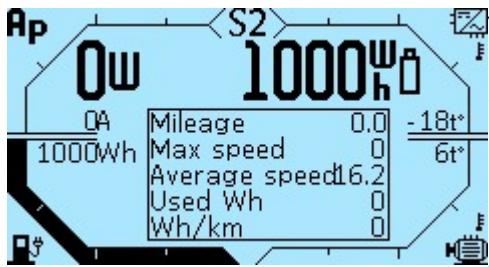
You can choose to display several types of statistics: **General**, **User**, **Trip**, **From charge**. For a detailed description, see the **Statistics** section. The main screen displays five parameters: **Mileage** — mileage in kilometers (**km**) or in miles (**mi**). **Max speed** — maximum speed, in kilometers per hour (**km/h**) or in miles per hour (**mph**). **Avg speed** — average speed, in kilometers per hour (**km/h**) or in miles per hour (**mph**).
