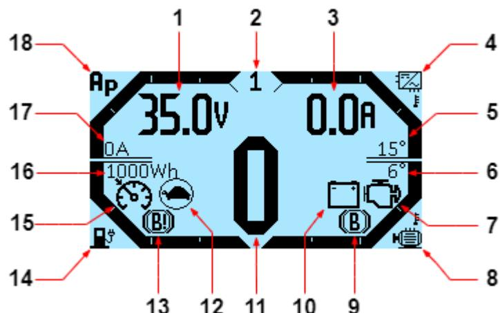
1. Information line, the content of which is changed by up and down keys. By default, the supply voltage is displayed in Volts (V). You can set up this line in the menu **On-board computer > Main screen setup > Information lines** (variable from the left side).
