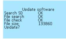
To update, download the firmware file to the root directory of the microSD card with Fat/Fat32 file system. Insert the card, with the contacts on top, into the connector on the On-board Computer. This can be done without turning off the On-board computer, but in this case, you must exit the **Firmware update** menu and reenter. After that, the On-board computer will detect the microSD card, display the **File size** in bytes and the menu item **Update**?
