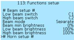
Next, select which button of the On-board computer the Low beam switch is connected to, we assigned the function **CAN**Separate select which button of the On-board computer the High beam switch is connected to, we assigned the function **CAN Button2** to the second button, need to select the value **C2**. It is impossible to assign the inclusion of low and high beam to one button, only to
