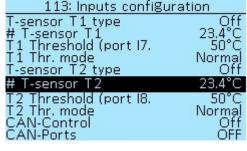
T-sensor T1 type — selection of NTC10K3950 or NTC10K3380 temperature sensor. Select Off if no sensor is connected.
