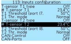
T-sensor T1 type — selection of NTC10K3950 or NTC10K3380 temperature sensor. Select Off if no sensor is connected.
