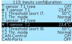
T-sensor T1 type — selection of NTC10K3950 or NTC10K3380 thermal sensor. Select Off if no sensor is connected.
