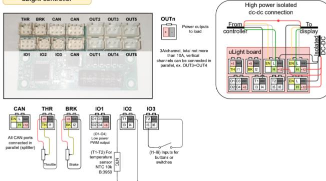
Connecting uLight to the Controller and the On-Board computer is possible in different ways:
