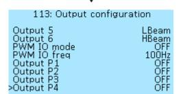
Output 1 — setting the function of output 1 (OUT1) of the uLight board. Selectable values — OFF (Disabled), ON (Always on), Bttn (Button, not yet implemented), TurnL (Left turn signal), TurnR (Right turn signal), Brk (Brake), LBeam (Low beam), HBeam (High beam), Rev (Reverse), Horn, TMot (Motor temperature), TCont (Controller temperature), T1 (External temperature sensor T1), T2 (External temperature sensor T2).
