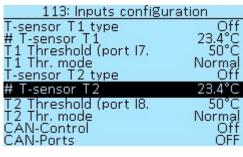
the **Function setup** section. Two thermal sensors can be connected to uLight. **T-sensor T1 type** — selection of **NTC10K3950** or **NTC10K3380** thermal sensor. Select **Off** if no sensor is connected.
