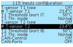
the **Function setup** section. Two thermal sensors can be connected to uLight.
