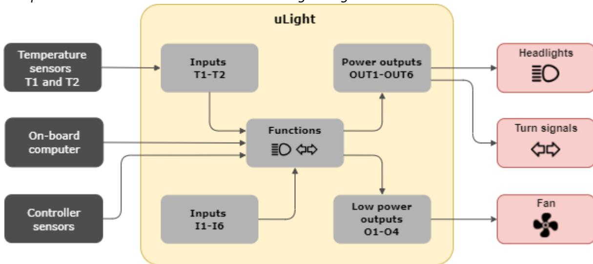
Setup ===== The uLight setup menu is located under **Settings > Devices > Nucular uLight**. Below you can find a detailed description of the menu items.
