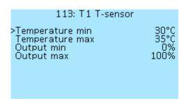
**Temperature min** — minimum temperature, values from -30 °C to 125 °C, in 5 °C increments. **Temperature max** — maximum temperature, values from -30 °C to 125 °C, in 5 °C increments. **Output min** — minimum output (PWM), values from 0% to 100%, in 5% increments. **Output max** — maximum output (PWM), values from 0% to 100%, in 5% increments.
