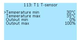
Temperature min — minimum temperature, values from -30 °C to 125 °C, in 5 °C increments.
