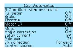
The auto-setup menu starts the subprogram and shows only the process. All settings are saved under **Controller** > **Motor setup**. After restarting the Controller, all switches will be in the **Off** position.
