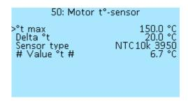
**\*t max** — maximum electric motor temperature, in degrees Celsius (\*C). Select of values from **50**°C to **200**°C, in increments of **1**°C.
