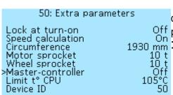
**Limit t° CPU** — limiting the temperature of the processor, in degrees Celsius (°C). When the specified threshold is reached, the phase current will be limited. Select of values from 60°C to 1930 mm 105°C, in increments of 5°C.
