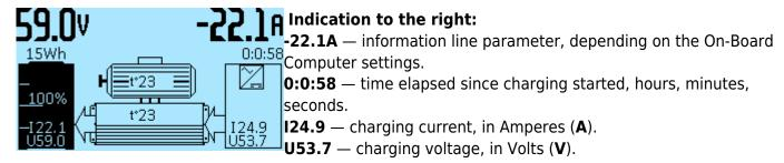
**The indication in the middle** is the temperature of the motor and the controller, respectively, in degrees Celsius (°C).
