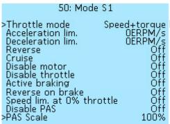
Throttle mode — selection of the operating mode of the throttle Speed+torque lever, read more in the section Throttle control mode setup.
