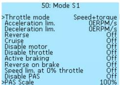
Throttle mode — selection of the operating mode of the throttle Speed+torque lever, read more in the section Throttle control mode setup.
