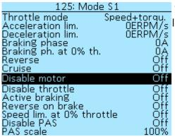
**Throttle mode** — selection of the operating mode of the throttle lever, read more in the section **Throttle control mode setup**.
