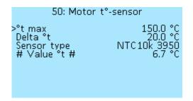
**\*t max** — maximum electric motor temperature, in degrees Celsius (\*C). Select of values from **50**°C to **200**°C, in increments of **1**°C.
