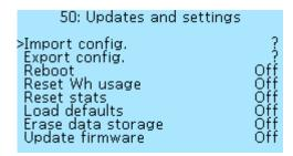
**Import config.** — loads the settings from the file **NCconf.cfg** - **NCconf9.cfg** up to a maximum of 9 different configurations, choosing a file number from 1 to 9. After a successful import, error messages may appear in the message, this means that not all the settings have been imported. In this case, it is advisable to check the downloaded settings with the original file by opening it in Notepad.
