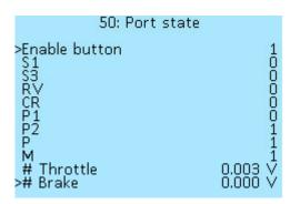
In the section **Controller** > **I/O configuration** > **Port state**, you can check input activation when contact shorted to GND. When a signal is applied, the value will change from **0** to **1**. Below in the menu items **# Throttle** and **# Brake** you can see the voltage on the throttle and brake levers, respectively.
