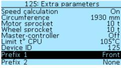
**Limit t° CPU** — limiting the temperature of the processor, in On 1930 mm degrees Celsius (°C). When the specified threshold is reached, the phase current will be limited. Select of values from 60°C to Off 105°C, in increments of 5°C.
