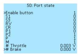
In the section **Controller** > **I/O configuration** > **Port state**, you can check input activation when contact shorted to GND. When a signal is applied, the value will change from **0** to **1**. Below in the menu items **# Throttle** and **# Brake** you can see the voltage on the throttle and brake levers,
