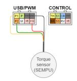
Pinout of controller ports
