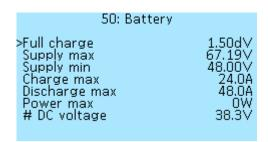
**Full charge** — delta voltage relative to the maximum, at which when the controller is turned on, will reset the watt-hour consumption, in volts (**dV**). This setting resets the **From charge statistics** when the Controller is turned on. Select values from **0.00 dV** to **10.00 dV**, in increments of **0.3 dV**.
