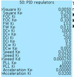
Two or three coefficients are used for the settings of each 0.0050 regulator: 0.250 **Ki** — integral coefficient.
