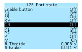
In the section **Controller** > **I/O configuration** > **Port state**, you can check input activation when contact shorted to GND. When a signal is applied, the value will change from **Off** to **On**. Below in the menu items **# Throttle** and **# Brake** you can see the voltage on the throttle and brake levers, respectively.
