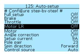
The auto-setup menu starts the subprogram and shows only the process. All settings are saved under **Controller** > **Motor setup**. After restarting the Controller, all switches will be in the **Off** position.
