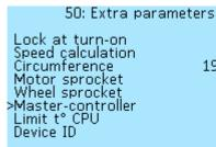
In the menu section **Controller** > **Extra parameters** > **Master**-Off **controller** you can enable the function of controlling other 1930 mm controllers from the current one. This setting is suitable for multi-10 t motor configurations where control (throttle, brake and etc.) is 10 t Off connected into one of the controllers directly. 105°C 50
