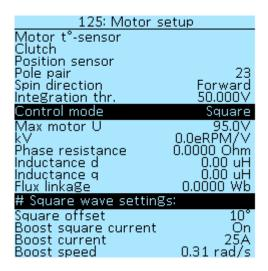
**Pole pair** — the number of pole pairs of the stator winding of the electric motor determines the speed at which the motor shaft will rotate. This parameter is used to calculate RPM and speed. For a more accurate autodetection of the Hall sensors angles, you must specify the correct value for the
