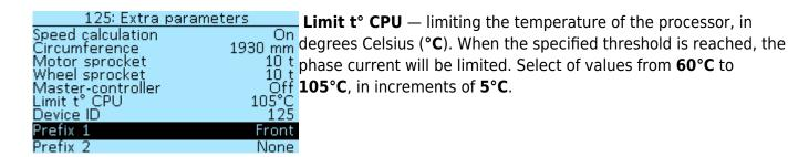
**Device ID** — setting the Controller number in the CAN network. This number is displayed in the menu section **Settings** > **Devices** in front of each device that is connected to the network using the **LEVCAN** protocol. If, by default, your device number is **0**, we recommend changing it to another
