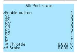
In the section **Controller** > **I/O configuration** > **Port state**, you can check input activation when contact shorted to GND. When a signal is applied, the value will change from **0** to **1**. Below in the menu items **# Throttle** and **# Brake** you can see the voltage on the throttle and brake levers, respectively.
