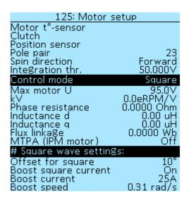
**Pole pair** — the number of pole pairs of the stator winding of the electric motor determines the speed at which the motor shaft will rotate. This parameter is used to calculate RPM and speed. For a more accurate autodetection of the Hall sensors angles, you must specify the correct value for the
