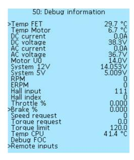
**Temp FET** — temperature of the field-effect transistors (MOSFETs) of the Controller, in degrees Celsius (°C).
