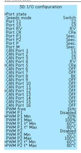
Available functions for the Controller ports S1, S3, RV, CR, P1, P2, P, M and CAN ports CAN port 1 -
