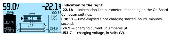
**The indication in the middle** is the temperature of the motor and the controller, respectively, in degrees Celsius (°**C**).
