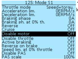
**Throttle mode** — selection of the operating mode of the throttle lever, read more in the section **Throttle control mode setup**.
