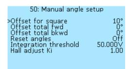
**Offset for square** — additional shift for square wave mode, in degrees (°). Select of values from -30° to 30°, in increments of 1°.
