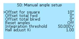
**Offset for square** — additional shift for square wave mode, in degrees (°). Select of values from **-30**° to **30**°, in increments of **1**°.
