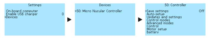
After configuring the battery, you need to run Auto-setup in the **Controller** > **Auto-setup** menu section. Ensure that the phase and battery wires are well contacted and insulated before running
